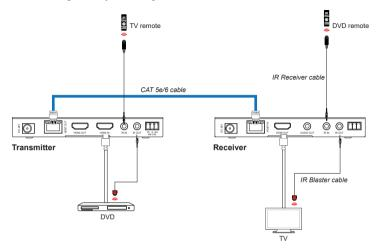
Note: When the angle between the IR receiver and the remote control is  $\pm$  45 °, the transmission distance is 0-5 meters; when the angle between the IR receiver and the remote control is  $\pm$  90 °, the transmission distance is 0-8 meters.
